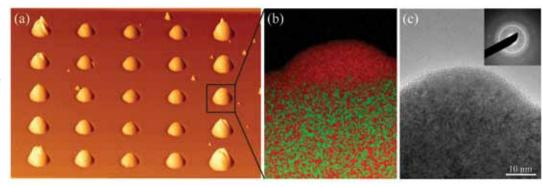
Figs: (a) AFM image of 2-dimensional FIB-fabricated Ga droplet array on GaAs; (b) XEDS cross-sectional map of Ga (red) and As (green) in the vicinity of a Ga droplet shows that the composition of this droplet is pure Ga; (c) cross-sectional TEM image and corresponding diffraction pattern in the vicinity of a Ga droplet indicate that the structure of the Ga droplet is amorphous and there is a polycrystalline GaAs layer underneath the droplet.
