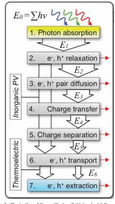
An illustration of the multi-step, light-to-electricity conversion processes for organic PV, inorganic PV, and thermoelectrics. The loss mechanisms at each step are also described.
